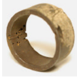
Figure 1 - Example of Pitting Corrosion
