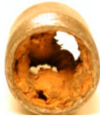
Figure 2 - Example of Tuberculation
