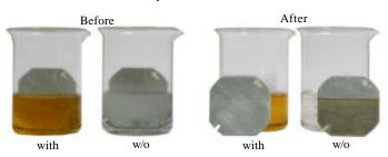
Note the prevention of damage to the galvanized sheet by CorroShield<sup>®</sup>
