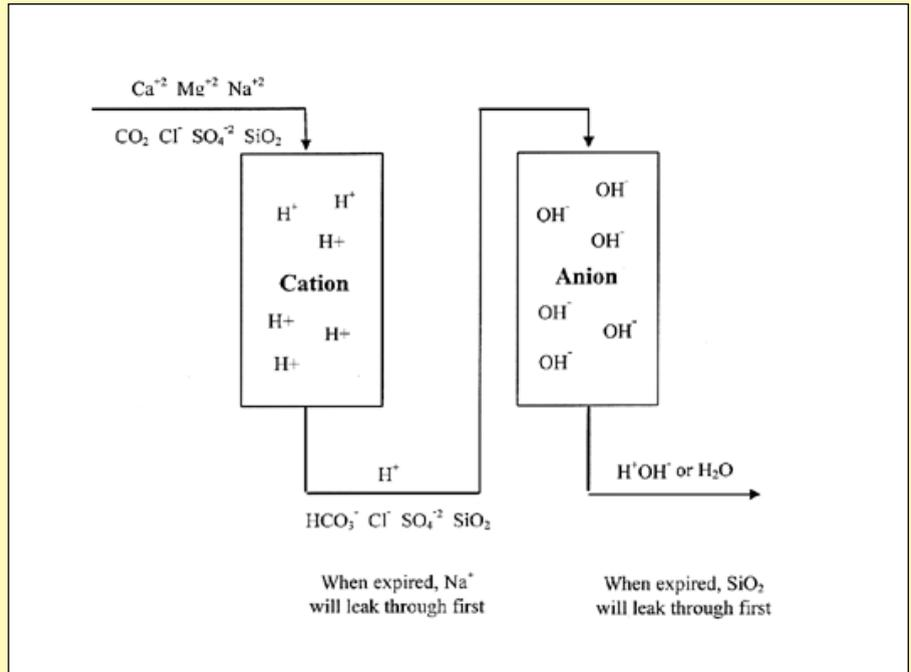
Figure 1 – Typical dual-bed deionizer
